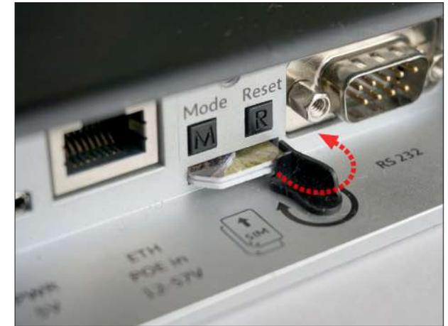
Rotate SIM card lock into position as indicated on above photo to lock both SIM cards.
