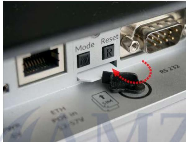
Rotate SIM lock to insert SIM card into slot.
