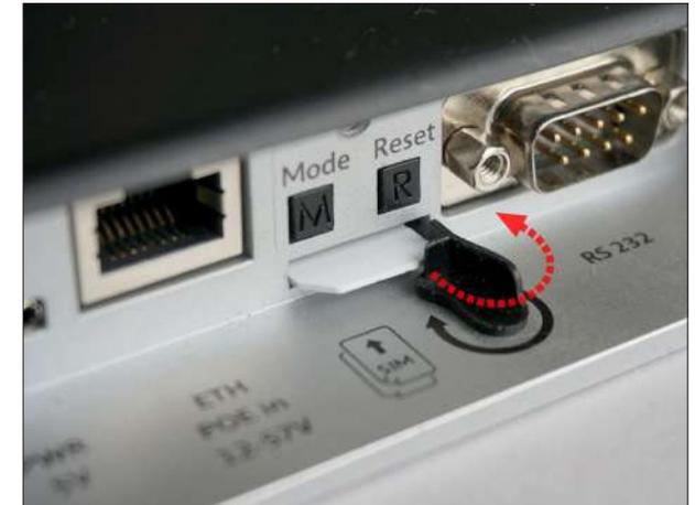
Rotate SIM card lock into position as indicated on above photo to lock SIM card.
