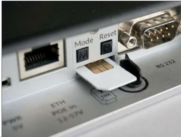
Position SIM card lock into position as indicated on a photo. Gently insert SIM card into lower slot.
