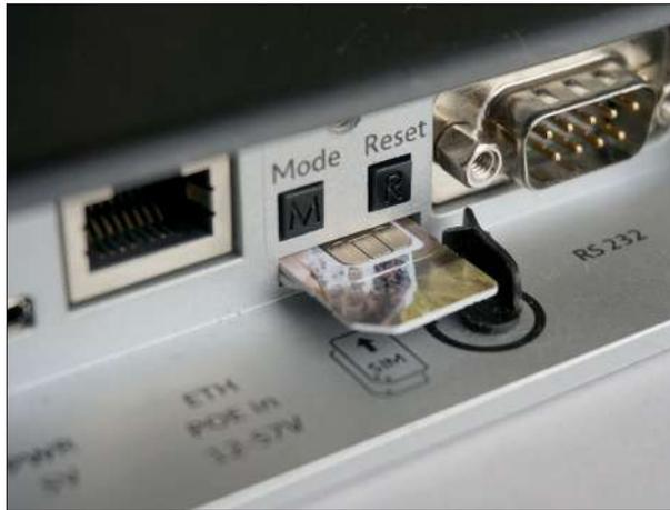
Position SIM card lock into position as indicated on a photo. Gently insert SIM card into upper slot.
